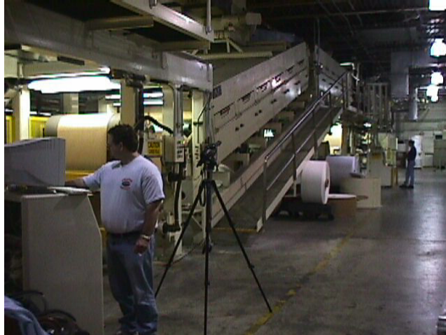
Figure 14 - Partial View of Pilot Coater Line. RKB Model 3030 was installed close to the take up reel. Paper is moving towards the left of this picture.
