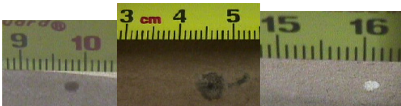
Figure 28 – Pictures of defects detected at production speed during the 33-lb Linerboard Export Test. Defects include a light spot, oil and type of scale
