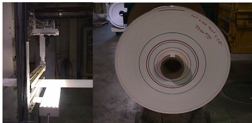
Figure 32 – View of inspection assembly during run and a picture of the Accolade Gloss Roll with defect location marks.
