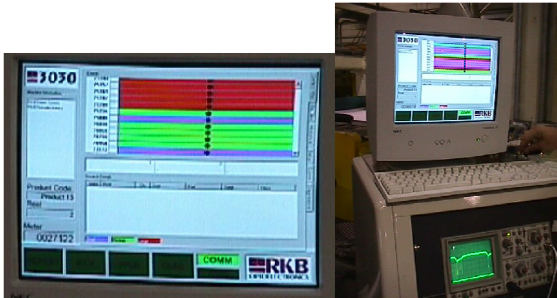
Figure 33 - View of cabinet and CRT screen during trial with calibrated defects. Each Red strip indicates a large size defect, Green medium and Blue small.
